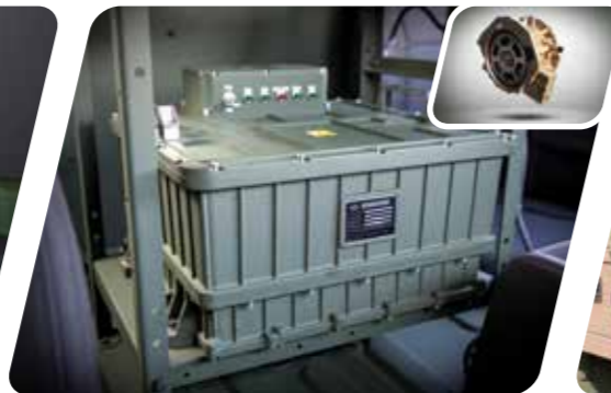
10kW Generator in Powertrain
