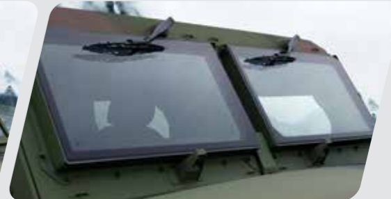
Bulletproof Windshield 2 piece glasses with defrosting heat film
